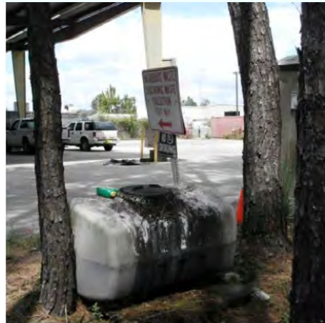
Photograph 3: HHW Collection Facility, High Priority Industrial Site Visit View of unprotected used household oil collection container with potential to contaminate nearby stormwater inlet
