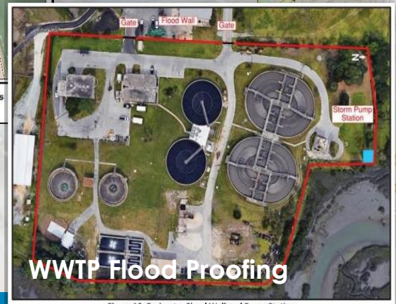
Figure 10: Perimeter Flood Wall and Pump Station
