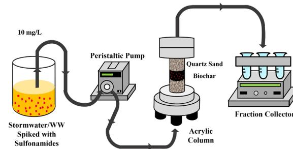
Schematic diagram of column filtration systems
