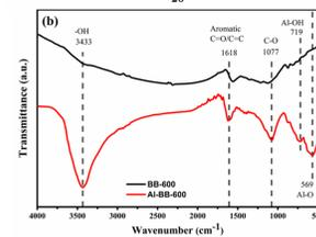
FTIR spectra of pristine biochar (BB-600) and Al-modified biochar (Al-BB-600)
