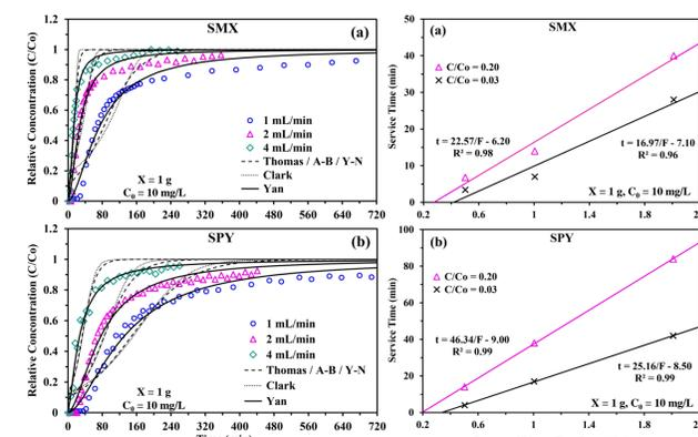
BT performance of (a) SMX, and (b) SPY under different flow rates.
