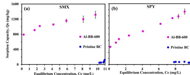
Adsorption isotherms of (a) SMX and (b) SPY onto pristine biochar and Al-BB-600 in wastewater.
