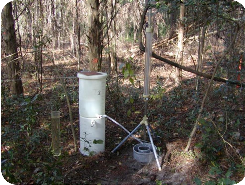
Predevelopment Infiltration Testing
