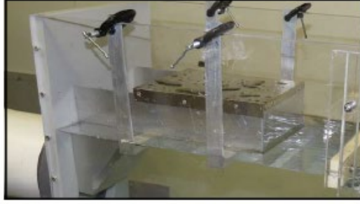
Model screen system is made from solid sheet metal.
