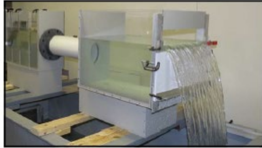
Tailwater vault simulates an adjacent elevated lake level.
