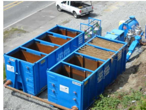
Sedimentation tanks with filter media
