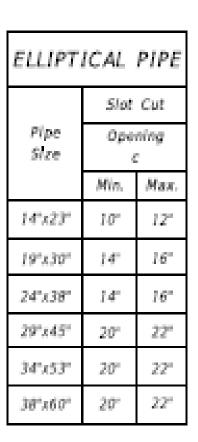
A curved cut is acceptable provided the control dimension is maintained (Typical For Elliptical & Round Pipe)
