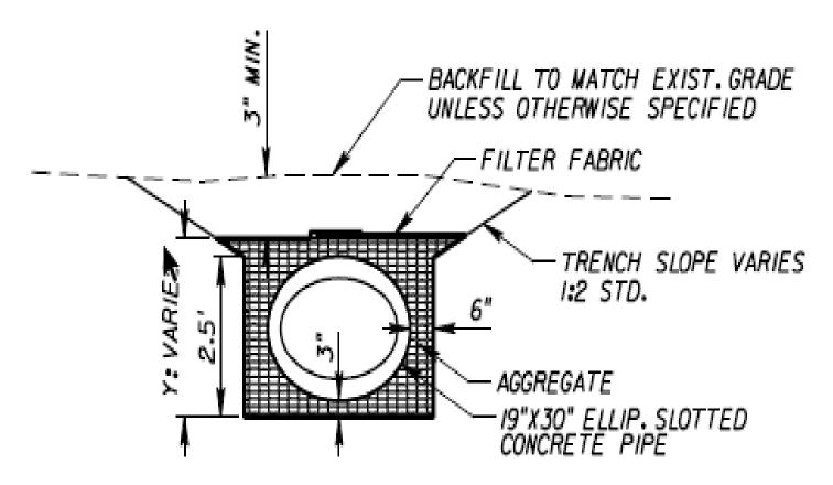
CONSTRUCT FRENCH DRAIN SYSTEM WITH THIS DETAIL AND INDEX 285, ALL NOTES AND DETAILS FROM INDEX 285 APPLY EXCEPT WHERE THEY CONFLICT WITH THIS DETAIL.
