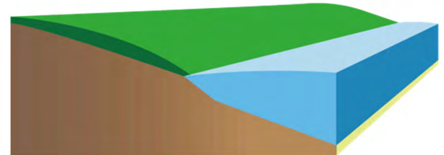
SOD OR PLANT DIRECTLY OVER THE SOX KNITTED MESH (CAN SOD ALL THE WAY TO THE WATERS EDGE)
