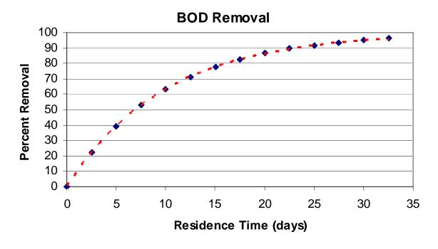
Figure 6-1. Theoretical Removal of BOD as a Function of Residence Time in a Wet Detention Pond.
