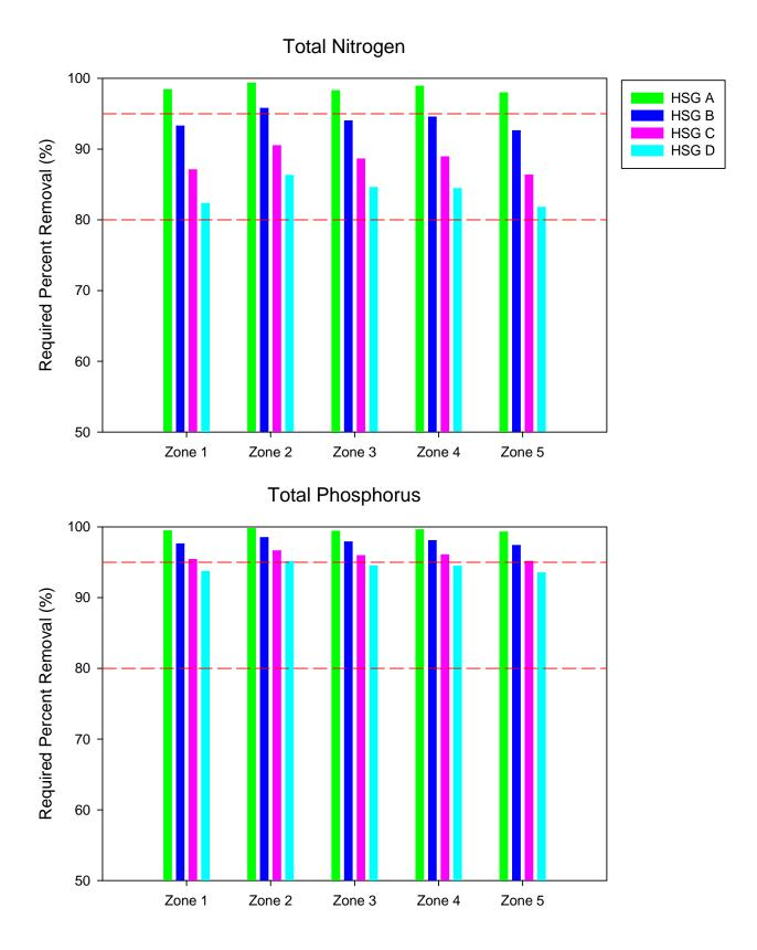
Figure 6-12. Comparison of Estimated Annual Mass Removal Efficiencies to Achieve Post-Development ≤ Pre-Development Loadings of Nitrogen and Phosphorus for a Highway (75% Impervious) Development.
