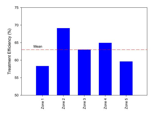
Figure 5-5. Calculated Annual Mass Removal Efficiencies for 0.5 inch of Dry Retention for a Development with 40% DCIA and a non-DCIA Curve Number of 70.
