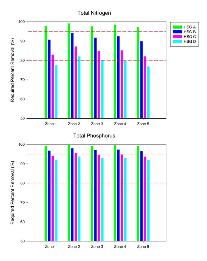
Figure 6-11. Comparison of Estimated Annual Mass Removal Efficiencies to Achieve Post-Development ≤ Pre-Development Loadings of Nitrogen and Phosphorus for a Highway (50% Impervious) Development.
