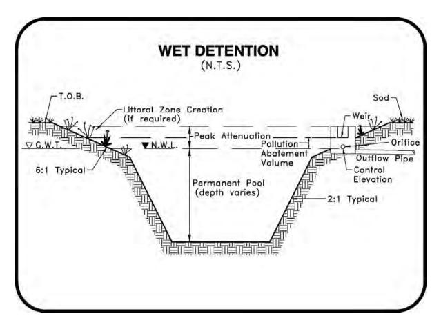
Figure 5-2. Schematic of a Wet Detention System.
