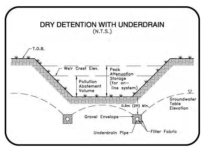
Figure 5-3. Schematic of a Dry Detention with Underdrain System.
