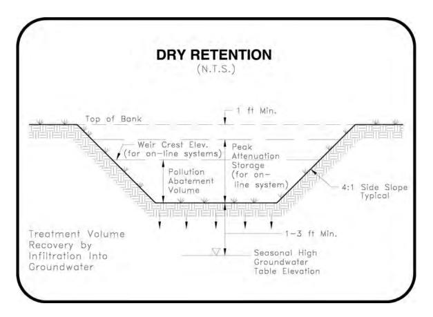
Figure 5-1. Schematic of a Dry Retention Facility.
