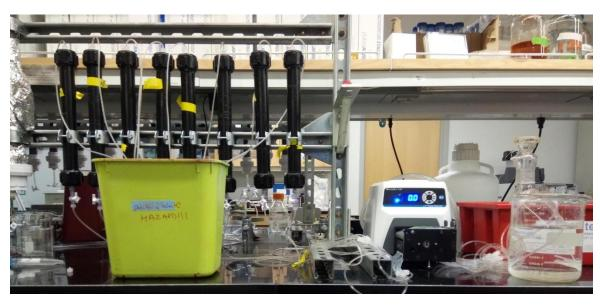
.Biochar was mixed with sand (70% by volume) and packed in a column (1 in ID x 12 in length). Stormwater contaminated with E. coli was injected.
